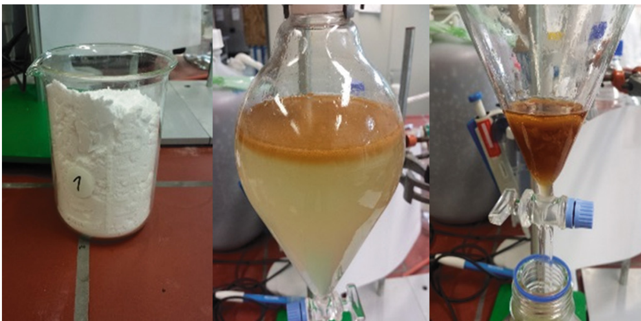
Downstream techniques have been developed in cooperation with Ostfalia University of Applied Sciences from Germany. Salting Out Extraction was tested for 2,3-Butanediol.
