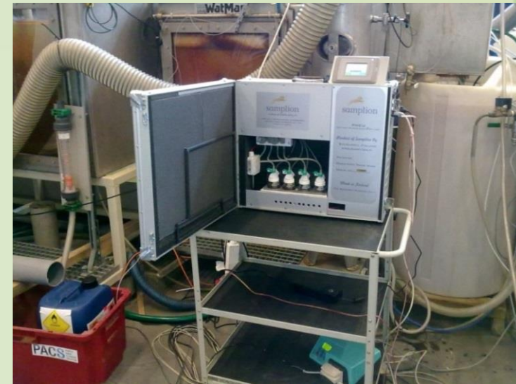
PMEU with Automated Sample Collection System
