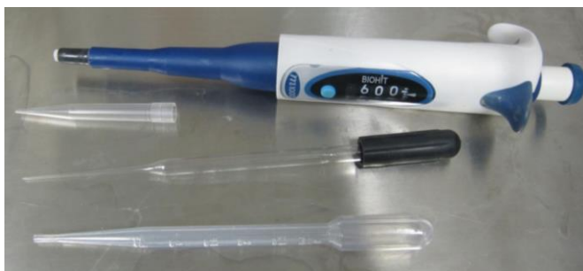
Picture 9. The uppermost is an automatic pipette and a tip for it. In the middle is a glass pasteur pipette and the last one is a plastic pasteur pipette.
