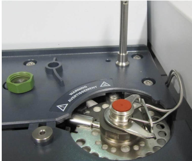
Picture 15. The soft and red part is a septum. If the side with a little hole in the middle of a septum is upwards, it has been set correctly.
