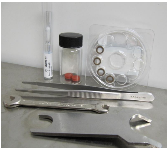
Picture 12. In the back, there is a liner, septums and o-rings from left to right. In front of them are tools for replacing them in the inlet and for maintaining the column.
