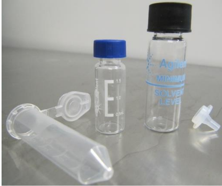
Picture 11. The first from the left is an eppendorf tube. Two others are vials; smaller one is for samples and bigger is for solvent and waste. The small thing in the right is a diffusion cap for a solvent vial.
