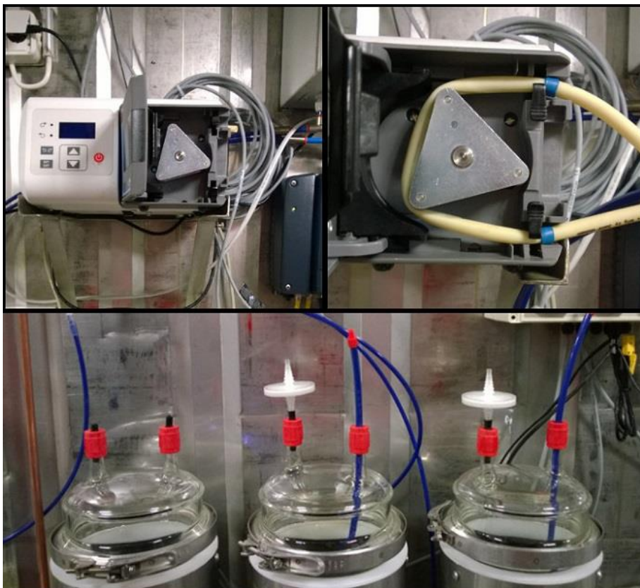
Picture 8 Hose pump and fermenters used to add microbiological mass to the bioreactor.
