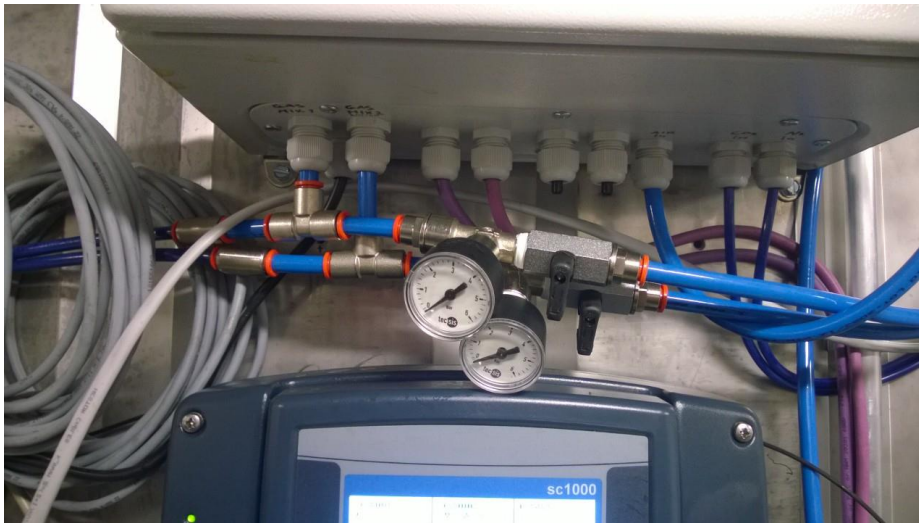
Fig. 5 Gas mixer outlets: pressure meters of each line (Reactor top and Reactor bottom).
