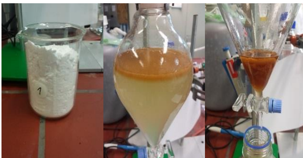
Figure 4: Salting out of 2,3-BDO from pre-cleaned fermentation broth. Water free K_2CO_3 (left), Formation of two layers in separatory funnel after K_2CO_3 addition, Contaminated 2,3-BDO phase with precipitated organic material.
