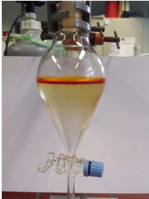
Figure 1: Separation of the two phases (2,3-BDO and water) after adding K_2CO_3 to the mixture. (2,3-BDO phase is colored with methyl red)
