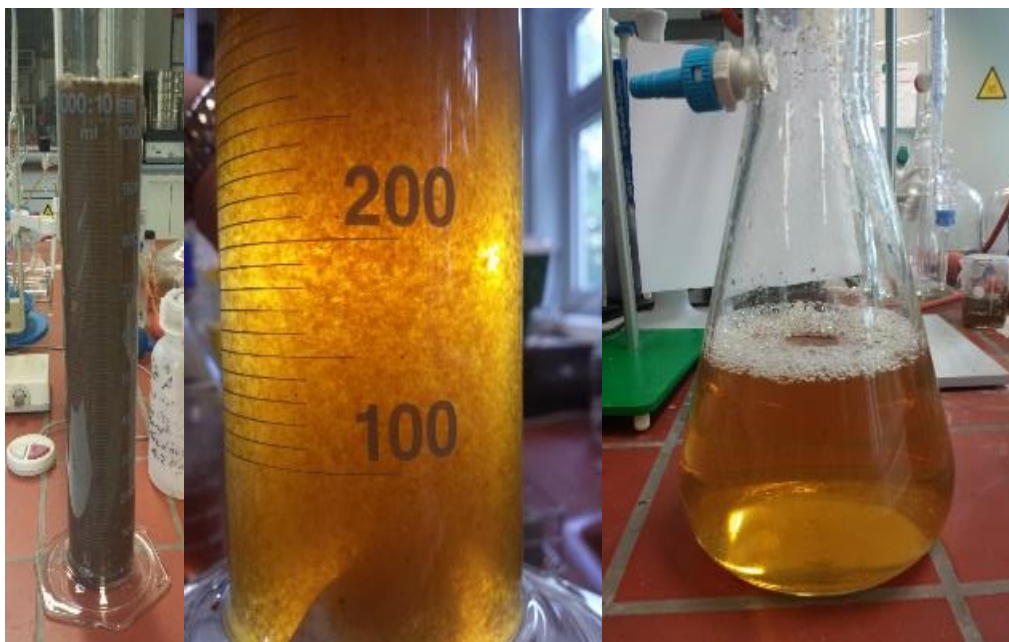
Figure 3: Pre-cleaning of the fermentation broth (left) by adding precipitation agent to the centrifuged solution (center). "Cleared" sample (right).
