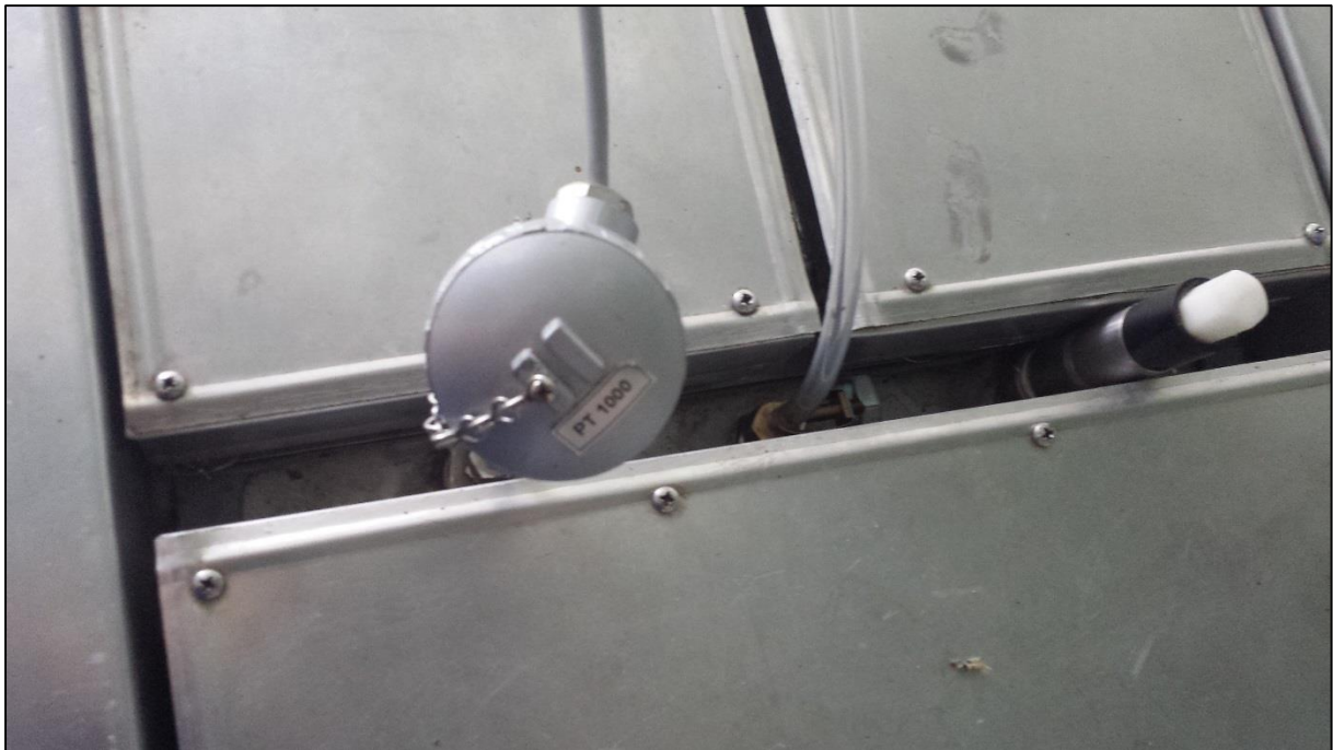
Figure 13: PT 1000 temperature sensor (foreground) and insulated covers (background). Spare mounting for temperature-/ pH-sensor (right) and gas inlet from the gas measurement system (center).
