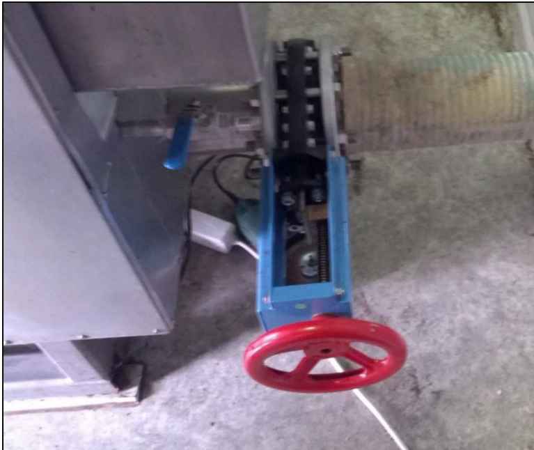
Figure 4: Main fermenter outlet DN 100. In the picture with a connected hose to drain the fermenter content.
