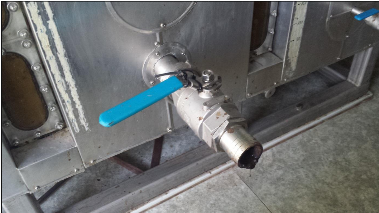
Figure 8: DN 50 ball valve for sampling of the fermenter content.
