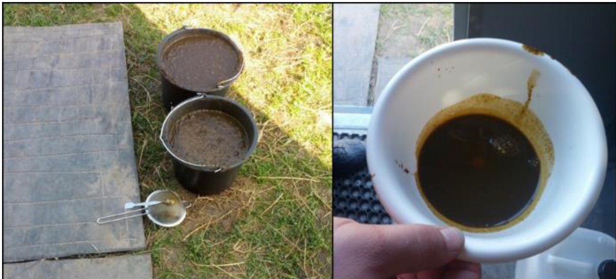
Figure 39: Samples taken from the fermenter. In the front a sieve to remove solid particles (left). Solid particles removed from the sample with the provided sieve (right).
