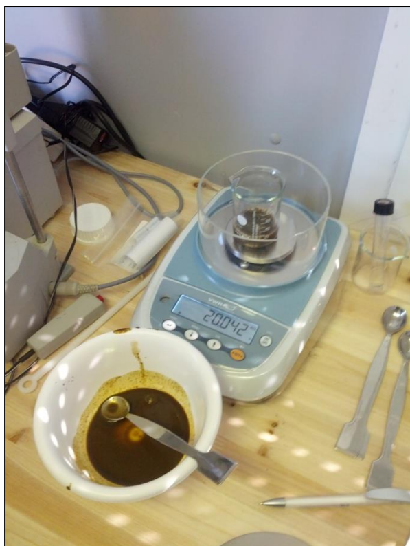
Figure 40: Sample preparation for VOA/TAC analysis.
