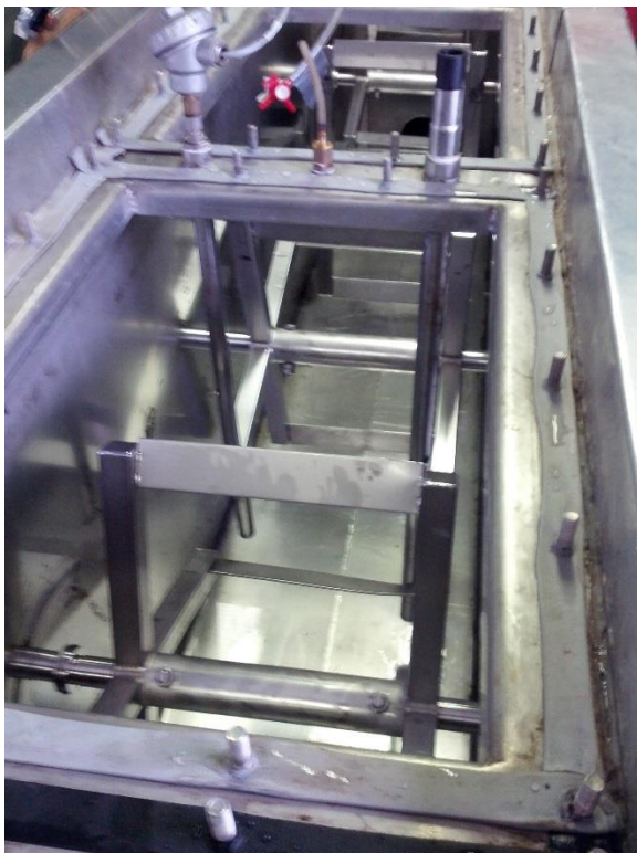
Figure 5: View on the agitators. Four of them are arranged horizontally over the length of the fermenter.
