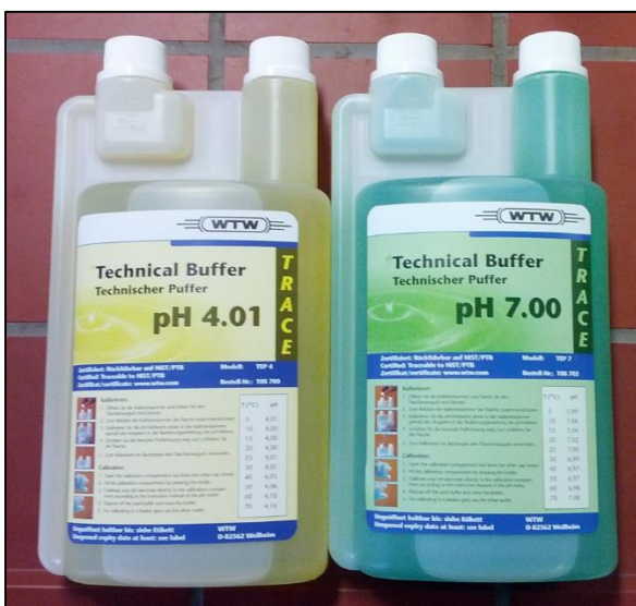
Figure 38: Buffer solutions pH 4.01 and pH 7.00 for calibration of the pH-electrodes.
