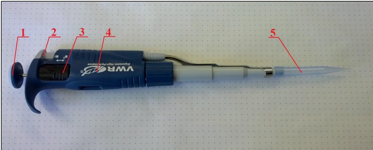
Figure 45: Precise dosing pipette with mounted disposable tip. (1) two-step button; (2) tip removal button; (3) dosing adjustment regulator; (4) dosing indicator; (5) disposable tip.
