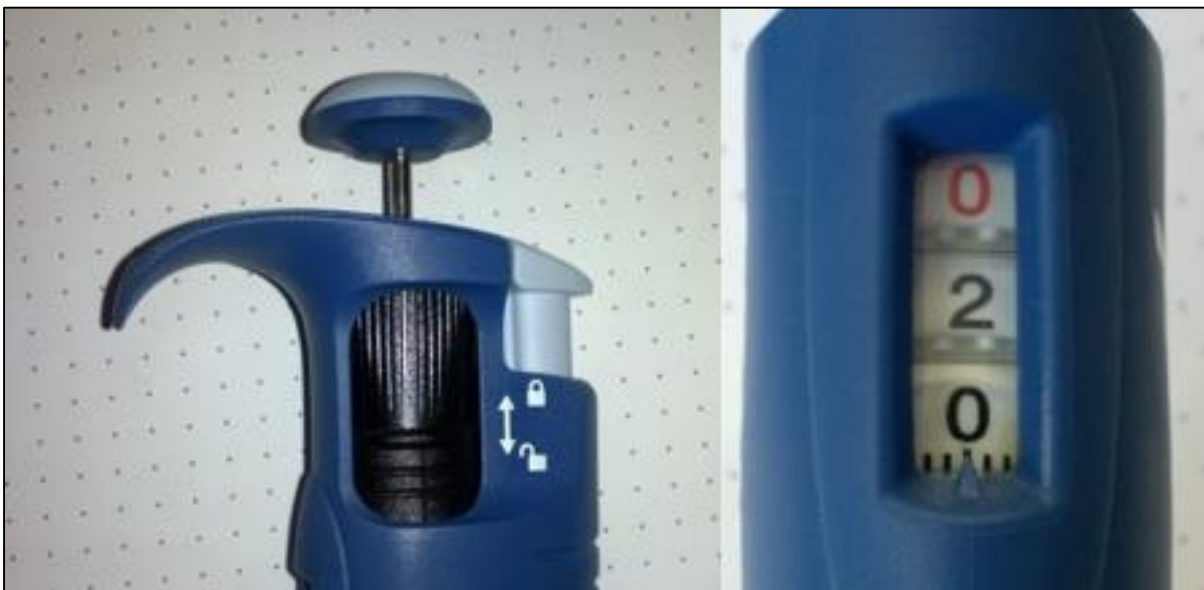
Figure 46: Pipettes adjustment example, with adjustment regulator (black) and adjustment value screen.
