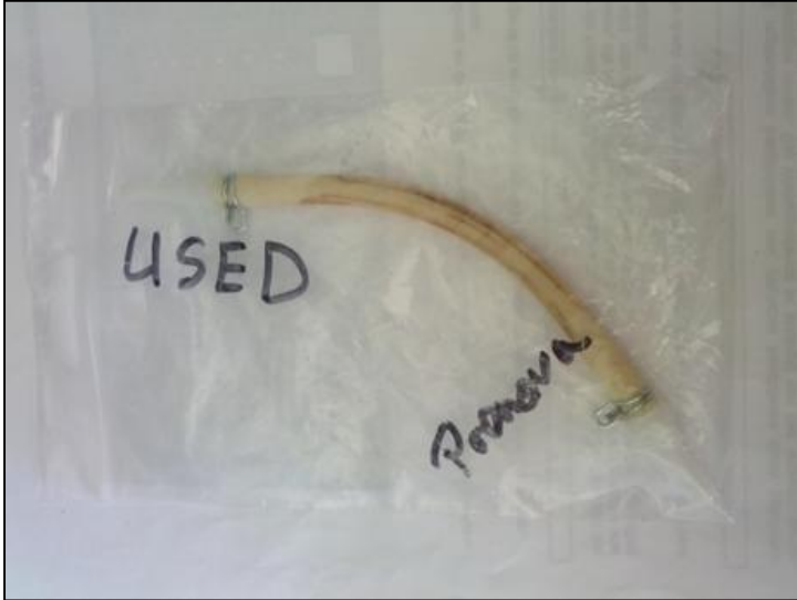
Figure 51: Rubber hose of the pump from the gas measurement system. Replaced due to wear marks/sounds.
