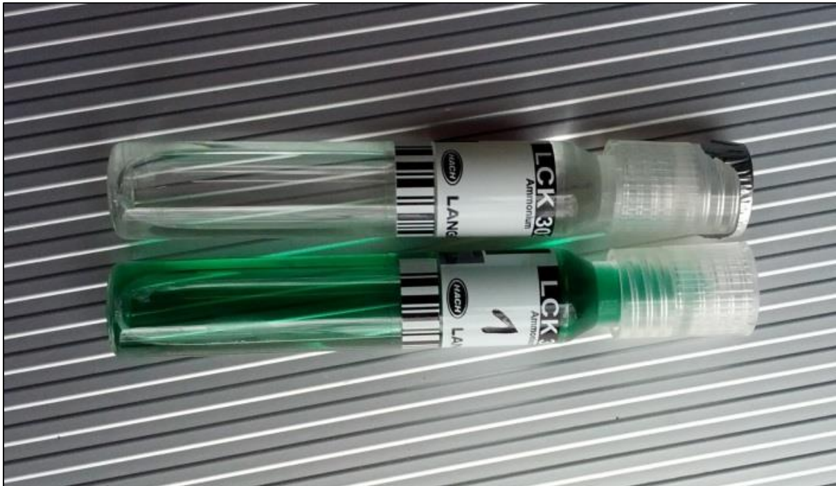
Figure 42: Dr. Lange LCK 302 cuvettes for ammonia analysis; cuvette with green liquid is already used, the one with the clear liquid is a new one.
