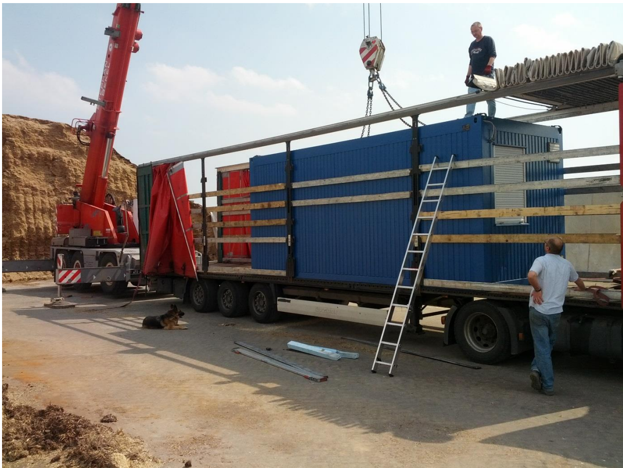
Figure 3: Loading of Pilot B in Germany. Difficult procedure because the container didn't fit through the top.
