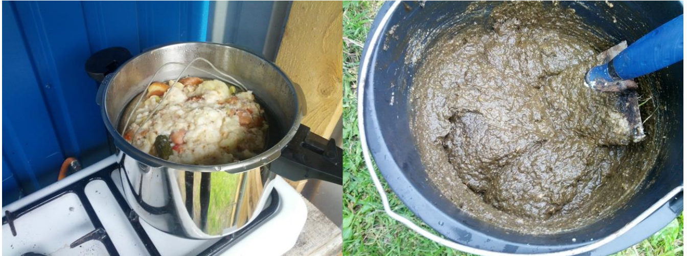
Figure 22: Sanitized food waste in pressure cooker (left) and premixed manure and food waste for fermenter feeding (right).
