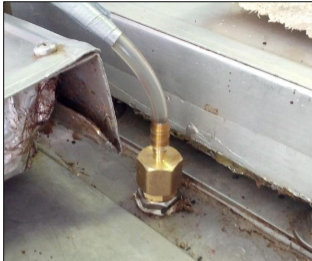
Figure 20: Exchanged gas in- and outlets to the gas measuring system.
