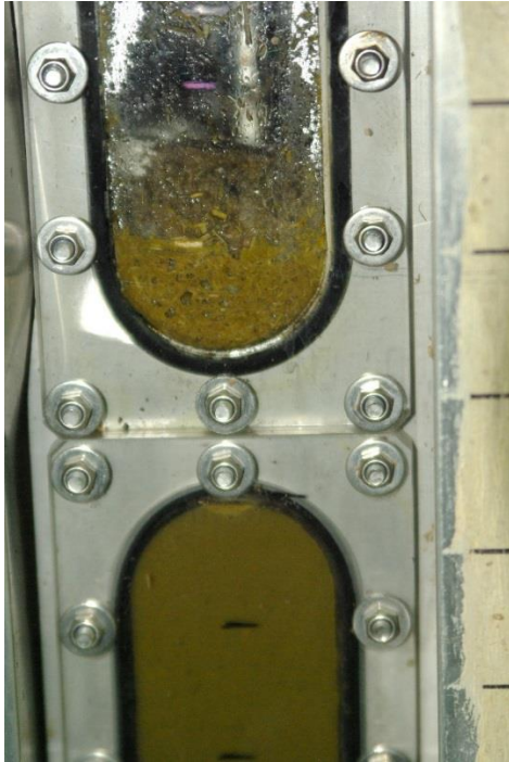
Figure 9: Floating layer forming in the fermenter contents surface.
