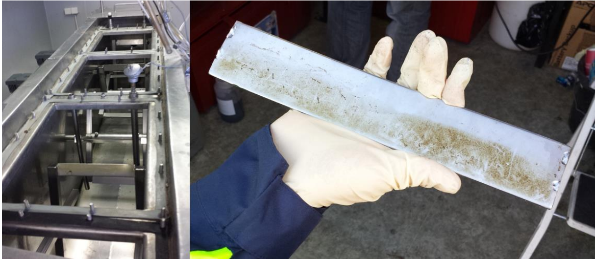
Figure 12: Broken stirrer paddle in pilot B
