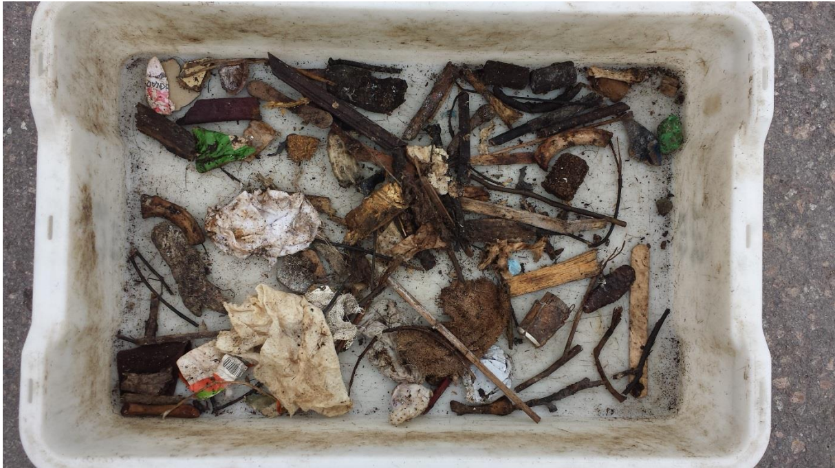
Figure 17: Sorted out fraction of organic matter; 13% of total mass sorted out; consisting of bones, wood pieces, cloth, cardboard, cork, and so on
