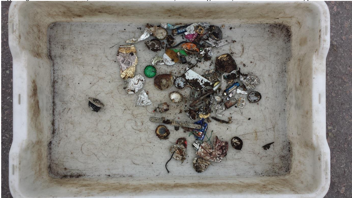
Figure 16: Sorted out metal fraction; 7% of total mass sorted out; consisting of metal and batteries
