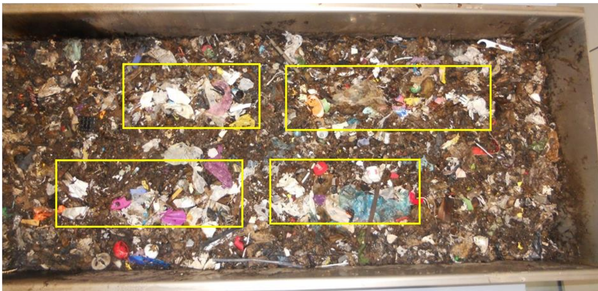
Figure 46: Residues in the container of the garage fermenter after first batch.
