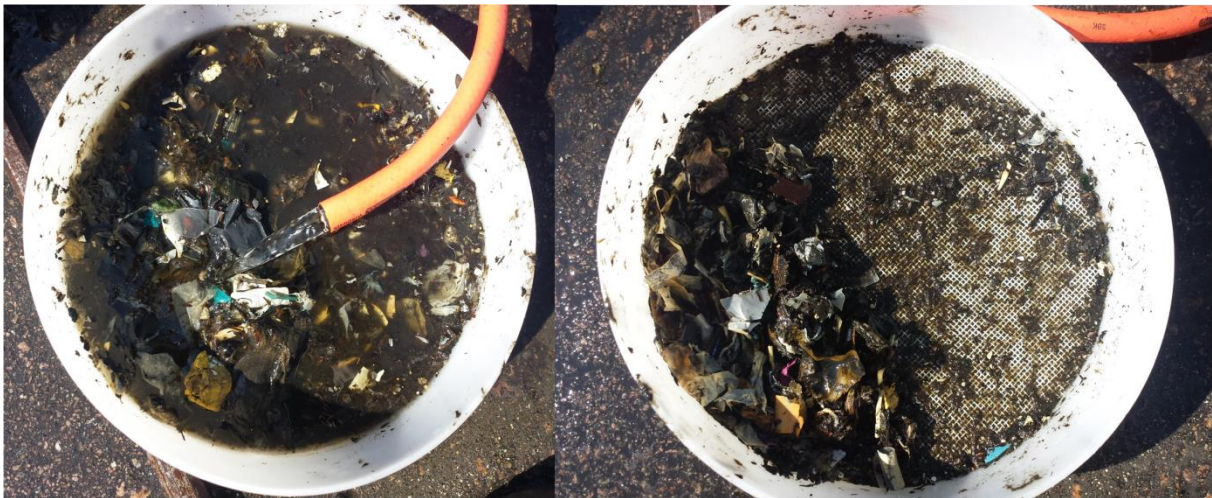
Figure 48: Impression of the residues after digestate washing.
