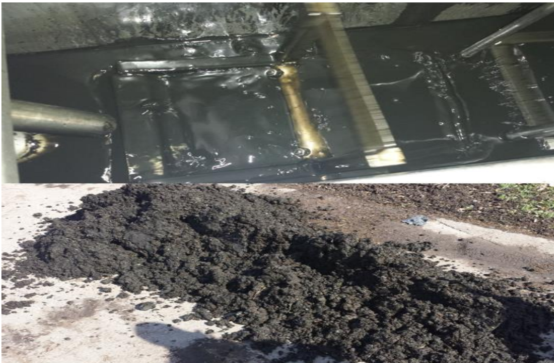
Figure 21: Initial filling of the fermenter. (Top) liquid digestate of the Växtkraft plant. (Bottom) solid digestate of the Växtkraft plant to adjust the dry matter content.
