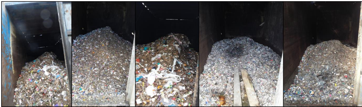
Figure 8: Impression of different MSW batches. The material has been shredded and sieved to a particle size \leq 30 - 40 mm.
