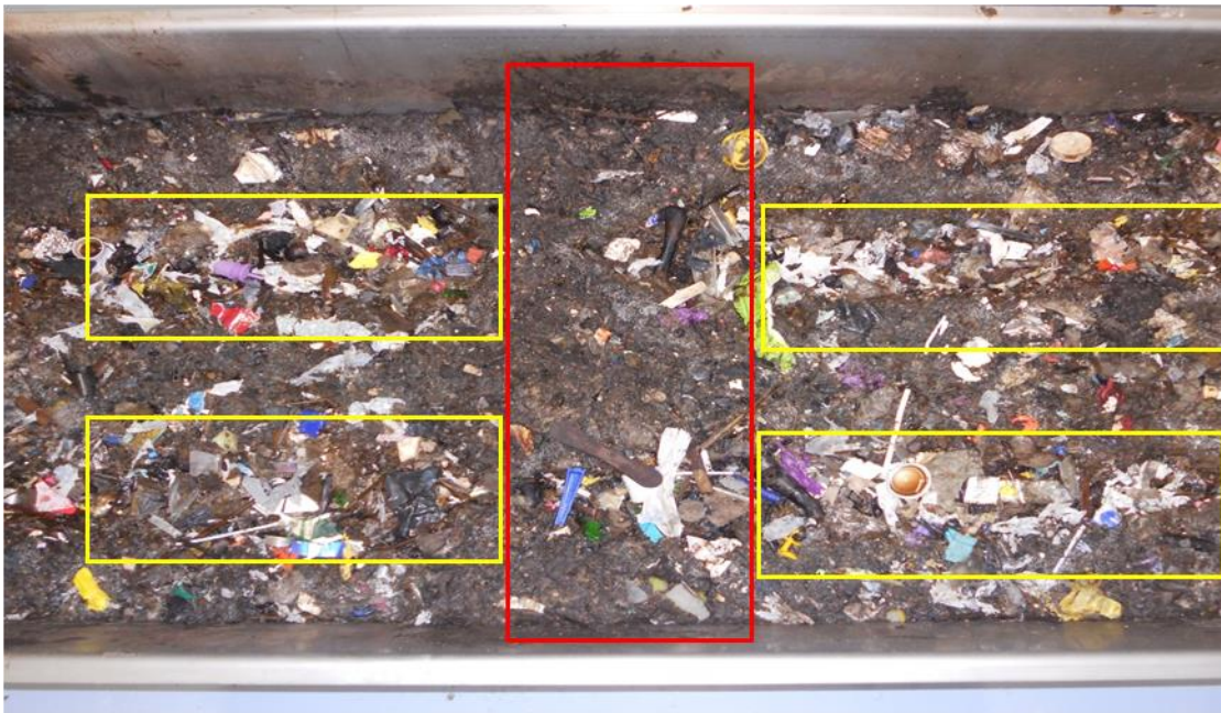
Figure 45: Residues in the container of the garage fermenter after
