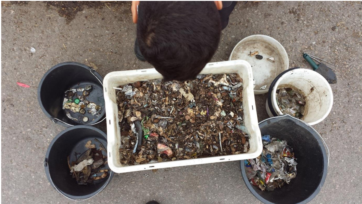
Figure 11: Sorting setup; exemplary sorting on 16 th July 2014 of waste to be fed to the fermenter
