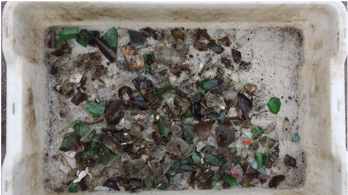
Figure 14: Sorted out glass fraction; 31% of total mass sorted out
