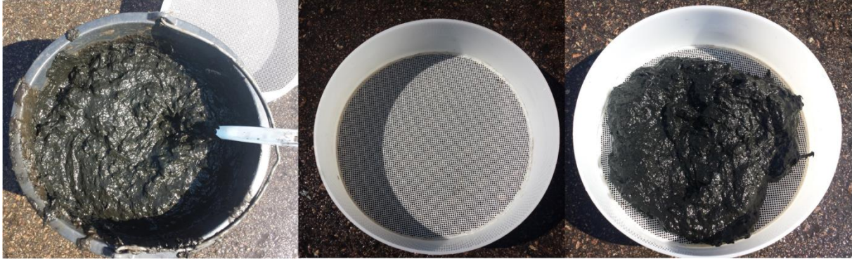
Figure 47: Leftovers after washing of the fermentation residues. 26% of digestate wet matter.
