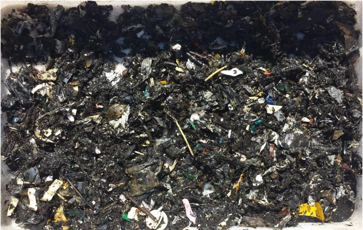
Figure 49: Residues after washing the digestate.
