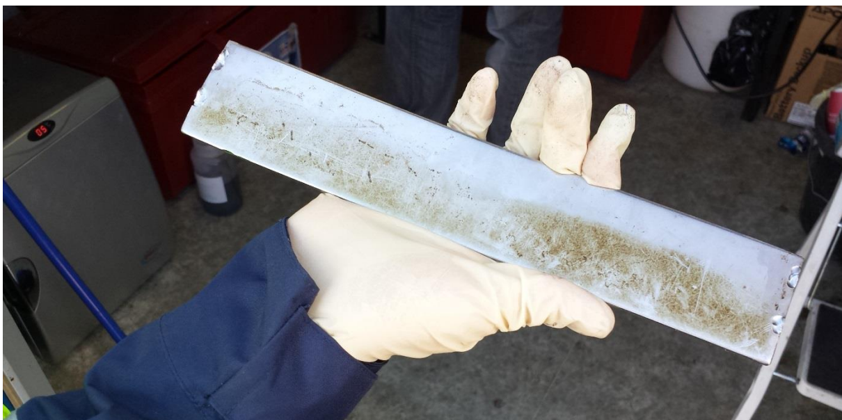
Figure 6: Broken paddle of the first stirrer.
