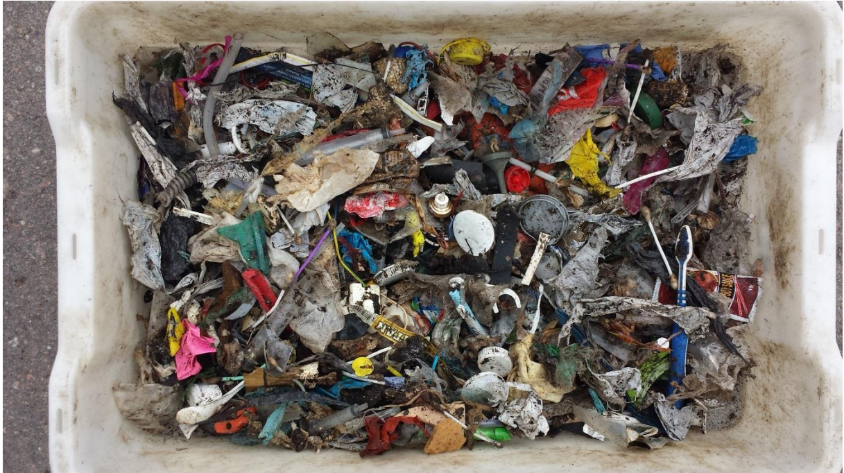
Figure 13: Sorted out plastic fraction; 41% of total mass sorted out; containing all kinds of plastic, rubber, foil, and so on
