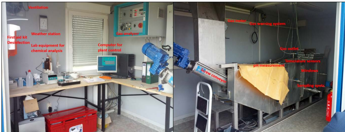
Figure 3: Interior of Pilot B Container. Left side: Laboratory, plant steering and measuring equipment. Right side: fermenter with technical equipment.
