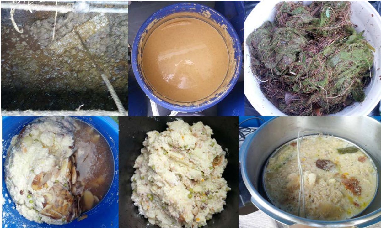
Figure 8: Substrates used in Lithuania. Cow manure (top left), Distillery leftovers (top middle), Algae (top right), Food waste (Original, mashed, sanitized) (from bottom left to right).
