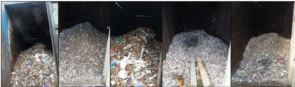
Figure 18: Different batches of MSW shredded and sieved to a size \leq 40 \text{ mm} . This has been the substrate used in Sweden.
